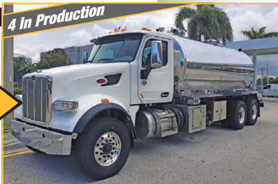
2019 Peterbilt 567, auto. trans., Cummins 450 hp, 4000/200 water alum. tank, PTO jetter w/ NVE 940 cfm blower
