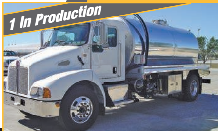
Kenworth T370, auto. trans., Cummins 300 hp., alum. 2500 gal., 320 cfm fan cooled pump
