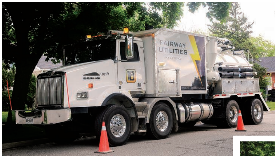
Left: The company's newest hydroexcavation unit, a Transway Systems Terra-Vex 125 built on a 2018 Western Star chassis, stands ready to work at a job site.
