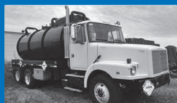
1994 Volvo WG64 with Presvac 3,300-gallon, two-compartment tank (2,300/1,000). Cat 3406, 400hp with Fruitland 1200 vacuum pump. .... $27,500 KLM Companies 617-909-9044 PBM
