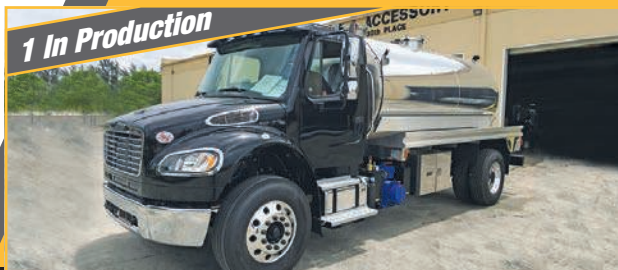
2019 Freightliner M2, Cummins 300 Hp. auto., 2500 gal. alum., fan-cooled Pump 320 cfm. chrome package
