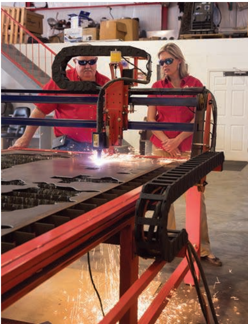
Above: Neal Bennett and Kimberly Bennett Wood work with a BurnTable computer numerical control plasma cutter to fabricate parts for a truck, including brackets and ladders.
