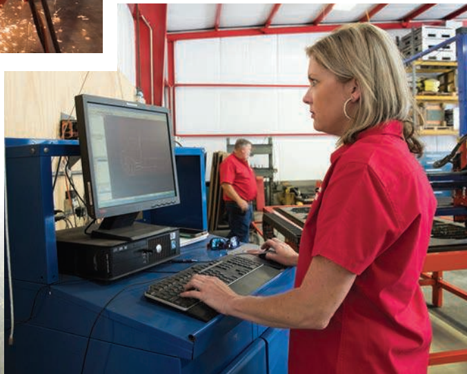
Above: Neal Bennett and Kimberly Bennett Wood work with a BurnTable computer numerical control plasma cutter to fabricate parts for a truck, including brackets and ladders.
