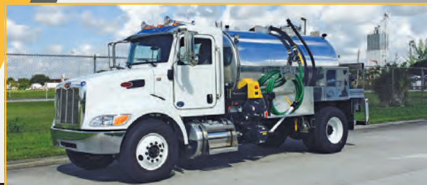
2019 Peterbilt 330, auto., 2000 alum. tank and Masport HXL4 vacuum system, the best working station on the market
