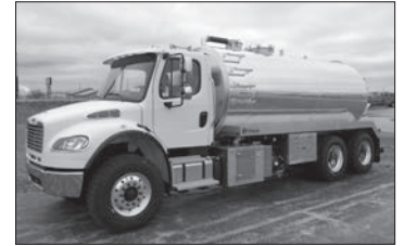
M2-106 with New 4000 Gal. Aluminum Imperial tank, NVE4307 Blower Package, 350 HP Cummins, Allison Auto., Full Lockers. Additional 4000 gal. tank units also available.
