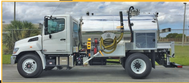
2019 Hino 268A with 2000 gallon tank and Masport HXL4 vacuum system
