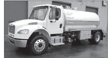
M2-106 with New 2500 Gal. Aluminum Imperial tank, NVE 607 Pump, Cummins L9 with an Allison 3000 RDS, Air Ride, Diff Lock. Additional 2500 gal. tank units also available.
