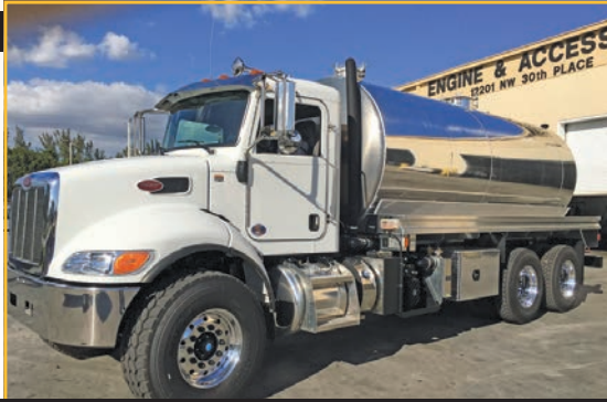
2019 Peterbilt 348 automatic transmission with NVE 4310 blower system, 940 CFM, 4200 alum. tank w/warranties
