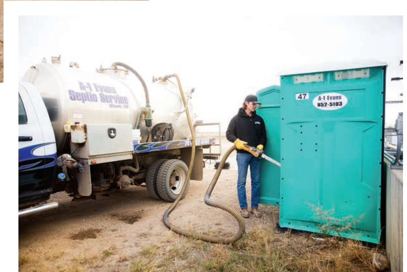
Below: Stopped at a construction site, Cole Ritter services a Satellite Industries Tufway restroom using a vacuum truck carrying a tank from Progress Tank and pump from Masport.
