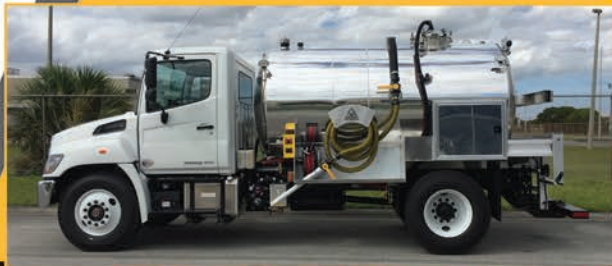
2018 Hino 268A with 2000 gallon tank and Masport HXL4 vacuum system
