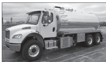
2018 M2-106 with New 4000 gal. Imperial Alum. Tank, NVE4307 Blower Package, 350 HP Cummins, Allison Auto., Air Ride, Full Lockers. 559763
