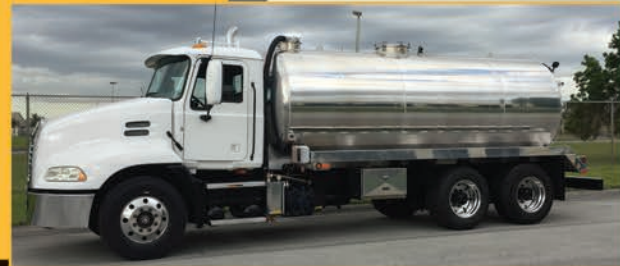
2011 Mack with New 3600 gallon tank and Masport Titan vacuum system
