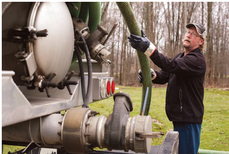
Technician Fred Bell puts away the hose to a 2006 Sterling built out by Mid-State Tank with a Jurop/Chandler pump after pumping a residential septic tank.
