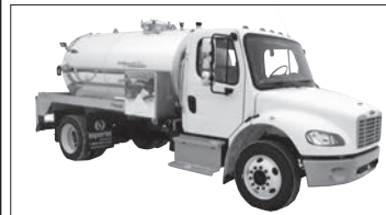
2018 M2-106 (non-CDL) with Imperial 2150 gal Alum. Tank, 1600 Waste/550 water Masport HXL75 Vacuum Pack., Cummins ISB w/Allison. 563468
