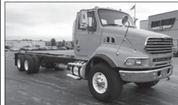
2007 Sterling LT9513, 410 HP, 4500RDS Allison Automatic, 20k Front Axle, 46k Rear Axles, Double Frame, Full Lockers. 574278
