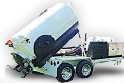
2016 Dodge 5500 Diesel (4 X 4), Auto, 1200 aluminum RVT, NVE 304 hydraulic drive pump package, DC10, two unit carrier.
