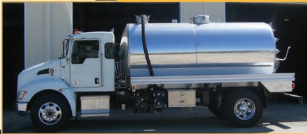
2018 Kenworth T370 Automatic transmission with 2500 gallon tank and Masport Titan vacuum system
