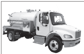
2018 M2-106 (non-CDL) with Imperial 2150 gal Alum. Tank, 1600 Waste/550 water Masport HXL75 Vacuum Pack., Cummins ISB w/Allison. 563468
