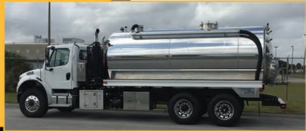
2018 Freightliner M2 with 4300 gallon tank, NVE 4310 Blower, 35 GPM Jetter
