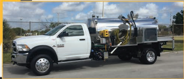
2017 Ram 5500 with 1500 gallon tank and Masport HXL4 vacuum system
