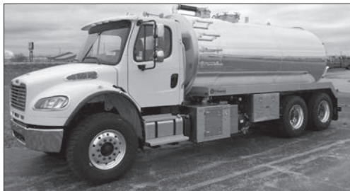
2018 M2-106 WITH NEW 4000 GAL. IMPERIAL ALUM. TANK, NVE4307 BLOWER PACKAGE, 350 HP CUMMINS, ALLISON AUTO., AIR RIDE, FULL LOCKERS. 559762, 559763
