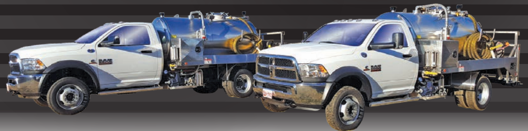
GH1100 800 waste/ 300 water mounted on a Dodge 5500
