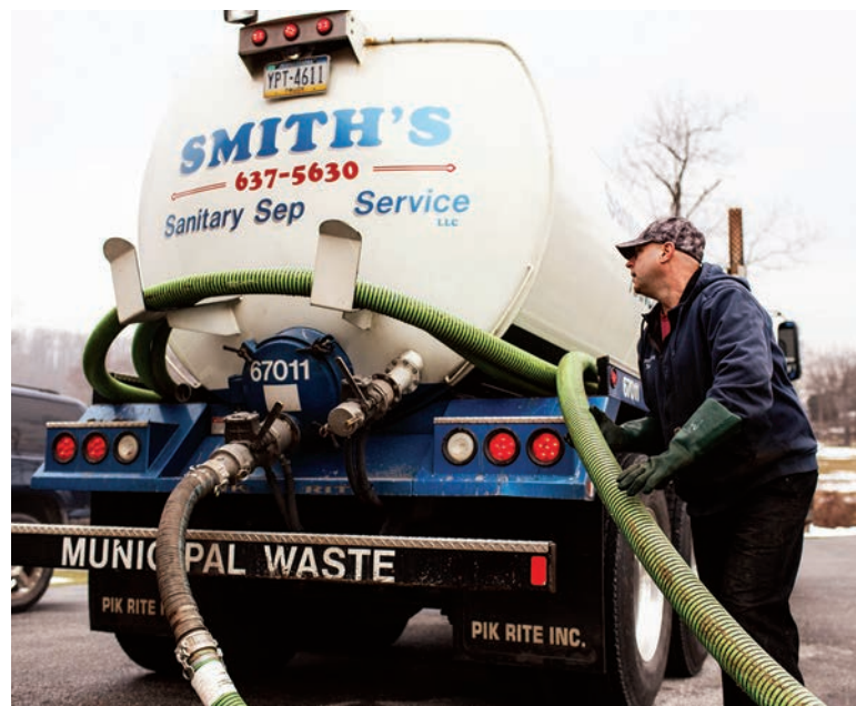
Above: Technician Todd Sherman racks the hoses after a residential pumping job. The truck was built by Pik Rite and uses a National Vacuum Equipment blower to generate vacuum.
