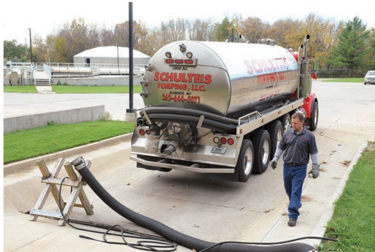
Left: Nate Hill readies his service truck for dumping. The rig is a 2005 Peterbilt 378 from T-Line Equipment with a 5,800-gallon tank and Masport pump.
