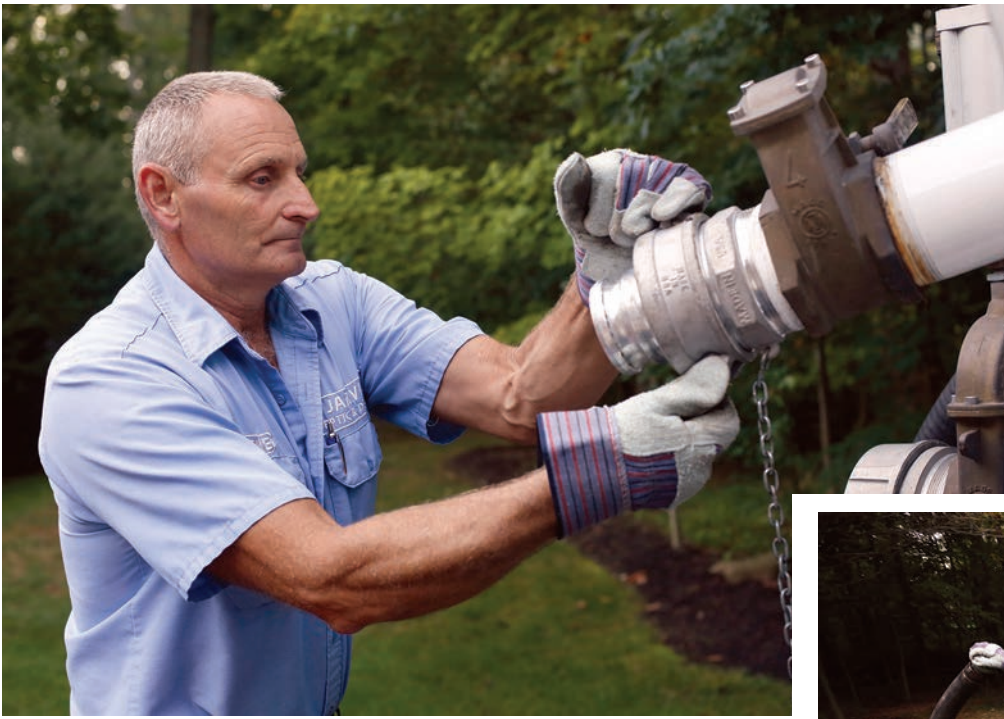
Left: Morris works a valve before hooking up his hose and pumping a septic tank.
