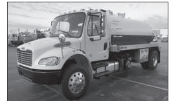
2008 M2-106 W/ New 2500 gal Imperial Tank, NVE 607 Pump, Mercedes and Allison 3000 RDS, Air Ride Suspension. 290892
