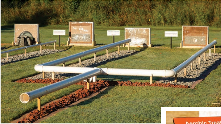
Above: Displays at the Onsite Wastewater Treatment Training Facility include cross-sections (at rear) so visitors have an idea of what the systems look like in the ground. (Photos courtesy Oklahoma State University)
