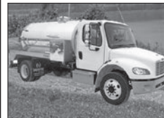
2018 M2-106 (non-CDL) with Imperial 2150 gal Alum. Tank, 1600 Waste/550 water Masport HXL75 Vacuum Pack., Cummins ISB w/Allison. Coming Soon!
