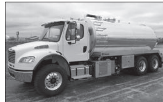
2018 M2-106 with New 4000 gal. Imperial Alum. Tank, NVE4307 Blower Package, 350 HP Cummins, Allison Auto., Air Ride, Full Lockers. Coming Soon!
