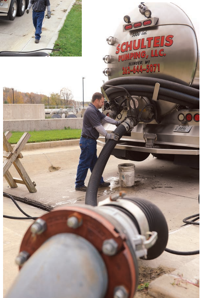
Below: The biggest vacuum truck in the fleet, with a 5,800-gallon tank, is capable of taking on loads from several septic tanks, and can handle large holding tanks and jobs from commercial customers. Here, Hill unloads at the local treatment plant.
