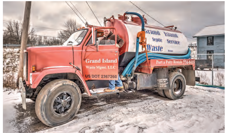
Below: Jim Ehde leaves for a run with the company's older rig, a 1985 GMC with a 2,500-gallon steel tank from Industrial & Municipal Engineering and a Pearson pump.
