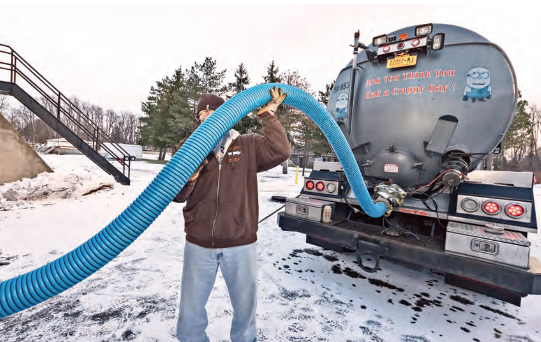
Left: Jim Ehde connects a suction hose at the Grand Island Water Pollution Control Center. The sludge will be hauled off the island to the Buffalo Sewer Authority for final processing.
