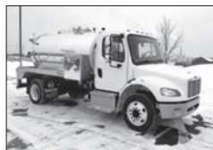
2017 M2-106 (non-CDL) with Imperial 2150 gal Alum. Tank, 1600 Waste/550 water Masport HXL75 Vacuum package, Cummins ISB with an Allison. 544718
