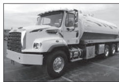
2016 114SD w/5000 gal Imperial Tank w/ NVE4307 Blower Package, Detroit DD13, Allison 4500RDS, 20K FA/46K RA w/Full Lockers. 391341
