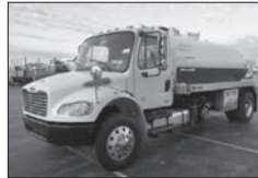
2008 M2-106 W/ New 2500 gal Imperial Tank, NVE 607 Pump, Mercedes and Allison 3000 RDS, Air Ride Suspension. 290892
