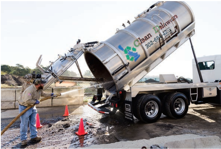
Above: Technician Chad Jones cleans debris from the tank of a 2014 Kenworth with a 4,200-gallon Presvac tank with NVE blower pump.
