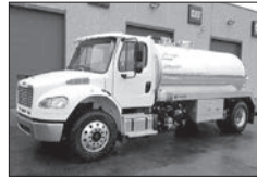
2018 M2-106 W/ 2500 gal Aluminum Imperial Tank, NVE 607 Pump, Cummins L9 with an Allison 3000 RDS, Air Ride, Diff Lock. 550250
