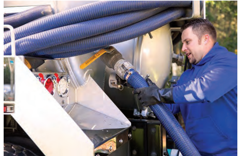
Below: Carlton hooks a suction hose in preparation for a pumping job.
