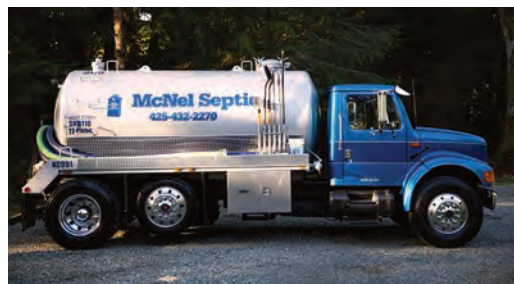
The company's clean backup pumping rig is a 1995 International 4900 with a 2,300-gallon steel tank, also built out by Erickson Tank & Pump with a Masport pump.
