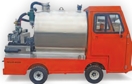
2017 Taylor-Dunn 500 gal. tank, NVE 866 pump package
