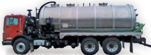
2010 MRU613 Mack 148K Mi., PR200 vacuum pump, 350HP, Allison 4500, NVE SS valves, 5200 gal. aluminum tank. Excellent condition.
