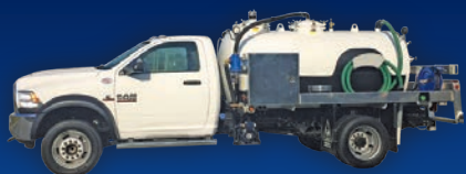
950 Gallon Portable Toilet Truck 2016 Dodge 5500, 950 Gal. Steel Tank
