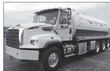
2016 114SD w/5000 gal Imperial Tank w/ NVE4307 Blower Package, Detroit DD13, Allison 4500RDS, 20K FA/46K RA w/Full Lockers. 391341
