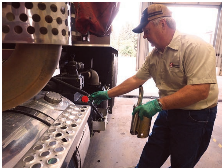
Below: Technician Art Betker adds oil to a Battioni pump on a Kenworth service truck built out by Friedrich's Auto & Truck.
