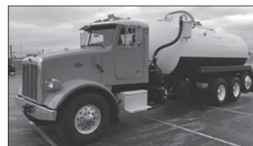
2003 Peterbilt 357 w/Newer 4500 gal. Tank, Cummins ISM, 20k Front and 46k Rears, Full Lockers, Low Hours. 544706
