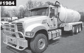
'12 MACK GRANITE GU713 MP8 @ 445 HP, Eaton-Fuller 13-Speed, 4,200 Gal. Steel Tank. $81,000.
