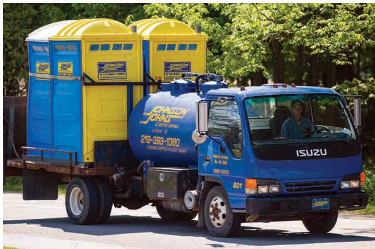
Above: Josh Ohime drives to a job site in his Isuzu service truck built in-house using a Conde (Westmoor Ltd.) pump and carrying four PolyJohn restrooms on the flatbed.
