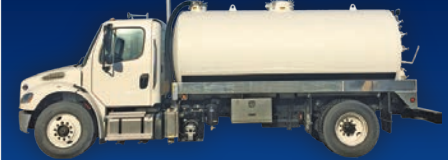
2500 Gallon Vacuum Truck 2016 Freightliner M2, 2500 Gal. Steel Tank
