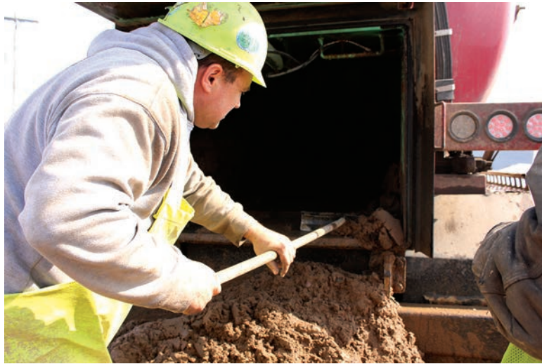
Below: Operator Kevin Schmoll shovels the remainder of the debris from a Premier hydroexcavator.
