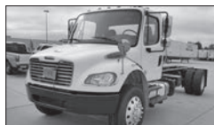
2011 Freightliner M2106, 325HP Cummins, Allison 3000 Series, Air Ride, New 2500gal Imperial Tank. 531894
