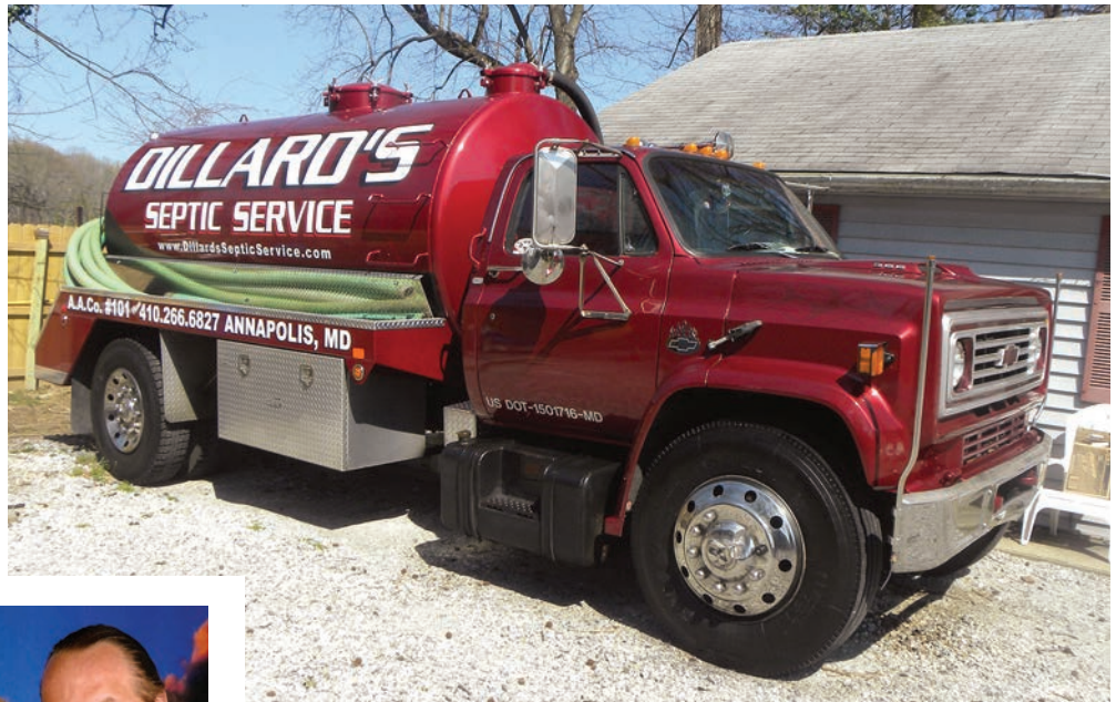
Above: Lely Manufacturing recently added a new tank and pump to James Dillard's 1988 Chevy vacuum truck. (Photos courtesy of James Dillard)
