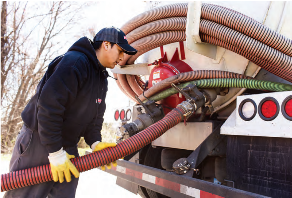
Left: Technician Nicolas Lema connects a vacuum hose to a service truck with an Imperial Industries tank and Masport pump.
