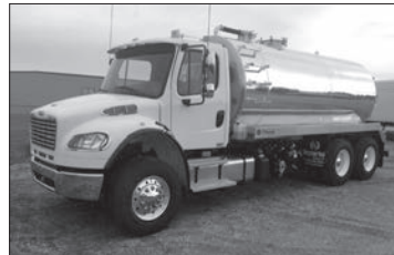
2016 M2-106 with New 4000 gal. Imperial Alum. Tank, 350 HP Cummins, Allison Auto., Air Ride, Full Lockers. 427239
