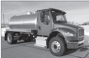
2016 M2-106 w/Imp. 2500 Gal Aluminum Tank, 380CFM Pump, 300HP Cummins ISL, Allison 3000RDS Auto., Air Ride Diff Lock. 395522
