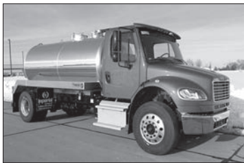
2016 M2-106 w/Imp. 2500 Gal Aluminum Tank, 380CFM Pump, 300HP Cummins ISL, Allison 3000RDS Auto., Air Ride Diff Lock. 395522
