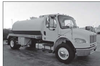
2007 M2 with New 2500 Gal. Tank, 360 CFM Pump, Mercedes 260 HP, Allison 3000 RDS Auto., Air Ride Cab and Suspension, Southern Truck. 418027
