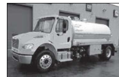
2017 M2 with 2500 Gal. Imperial Tank, 380 CFM Pump, 300 HP ISL Cummins, Allison 3000RDS Auto., Air Ride, Diff. Lock. 434003
