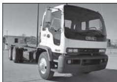
2002 GMC T8500, 250 HP Cat, 54,600 pound GVW, Allison Automatic w/PTO Cap., Double Frame, Hendrickson Suspension. 409870
