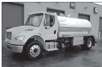
2016 M2 with 2500 Gal. Imperial Tank, 380 CFM Pump, 300 HP ISL Cummins, Allison 3000RDS Auto., Air Ride, Diff. Lock. 395522
