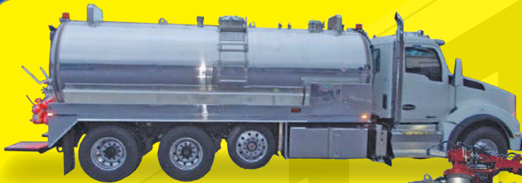
Aluminum 2 Compartment With Jetter System
