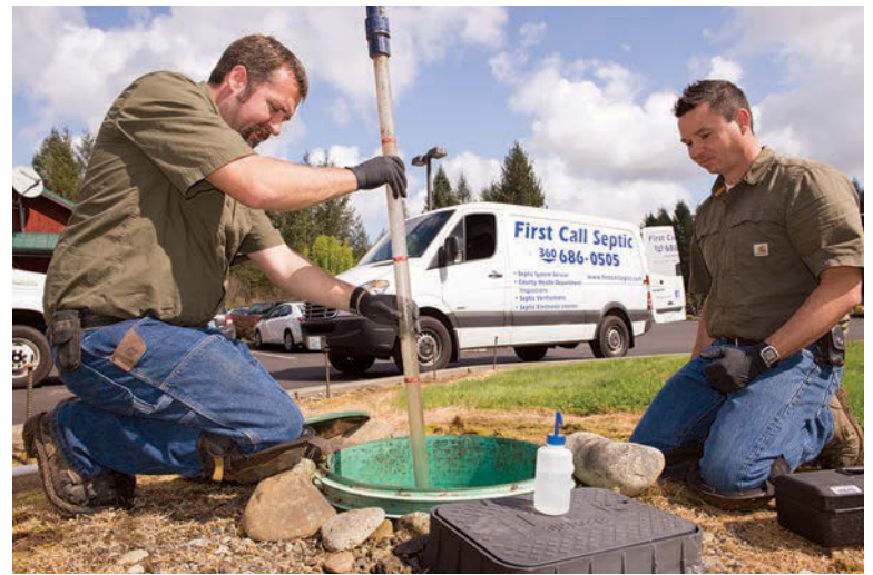
Below: Tamez, right, and Gross use a Sludge Judge during the inspection of a commercial septic system at a local business in Battle Ground, Washington.
