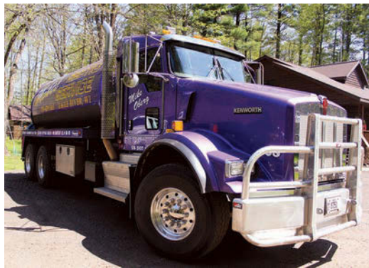
Below: Kenworth is the preferred truck brand and purple is the distinctive company color for Mike’s Septic Service, in Eagle River, Wisconsin. Here technician Ike Roberts backs a 2012 rig built out by Imperial Industries with a Masport pump toward a residential septic tank for pumping.
