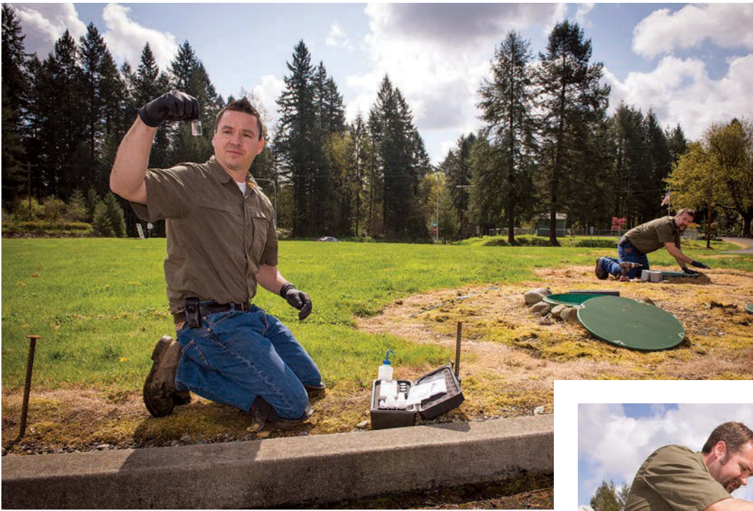
Left: First Call Septic owner Ronnie Tamez takes an effluent sample during an onsite system inspection while technician Chris Gross works in the background.
