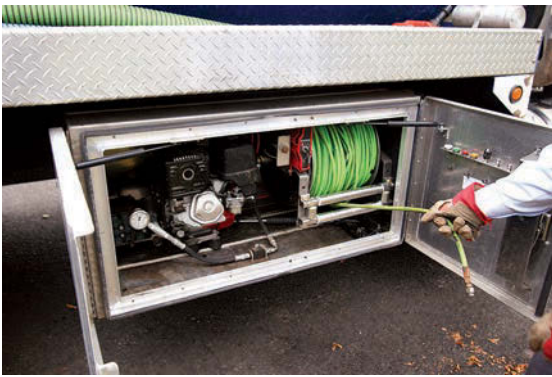
Mounted below his truck's hose tray, a toolbox jetter from Advance Pump & Equipment comes in handy to clear a clogged line during a maintenance call.
