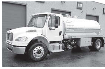
2016 M2 with 2500 Gal. Imperial Tank, 380 CFM Pump, 300 HP ISL Cummins, Allison 3000RDS Automatic, Air Ride, Diff. Lock. 395517
