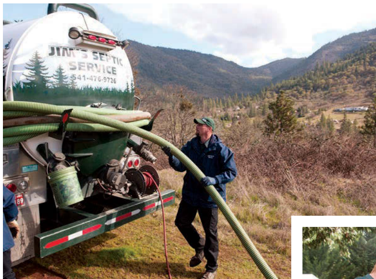
Left: Technician Joshua Fiske works in some beautiful Oregon territory. Here he returns a hose to his pumping rig, a 2006 Freightliner with a National Vacuum Equipment pump from House of Imports.
