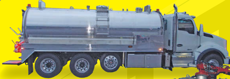
Aluminum 2 Compartment With Jetter System
