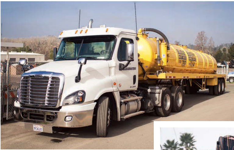
Above: Sludgebusters is constantly updating its fleet of trucks. This new rig, a 2015 Freightliner with a Battioni pump and a 5,460-gallon tanker from Mid-Continent Truck Sales and Bird Tank, is used for large pumping jobs and waste storage.
