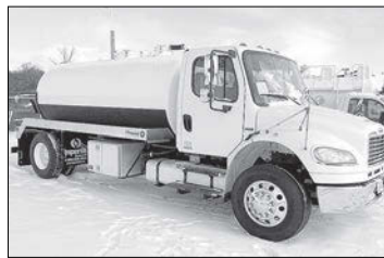
2008 M2 with New 2500 Gal. Tank, 350 CFM Pump, Cummins ISC 260 HP, Allison 3000 RDS Auto., Air Ride Cab & Suspension, Southern Truck. 410491
