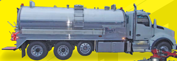
Aluminum 2 Compartment With Jetter System
