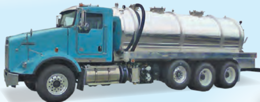
2015 Kenworth, tri-axle 4200(200/4000) NVE Challenger 866, jetter system.
