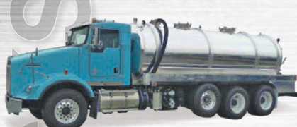
2015 Kenworth , tri-axle 4200(200/4000) NVE Challenger 866, jetter system.
