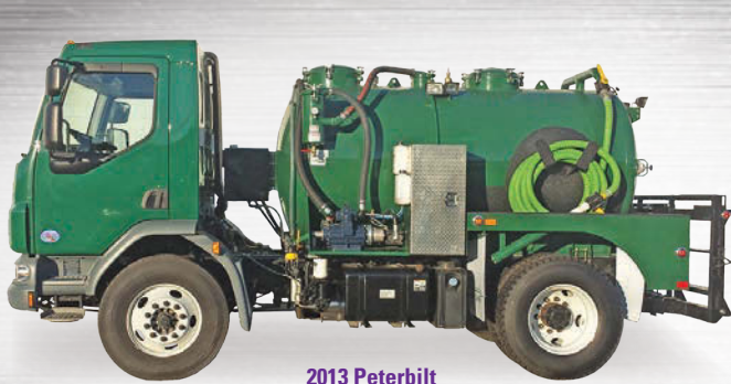
2013 Peterbilt 26,000 GVWR, auto transmission, 400/1100 stainless steel tank, Masport HXL4 pump, dual service-loaded.
