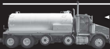
2005 Kenworth with 4600 gallon tank, Masport HXL400 pump
