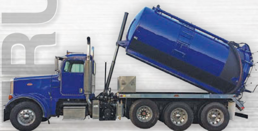
Peterbilt 4500 gallon stainless, hoist tank
