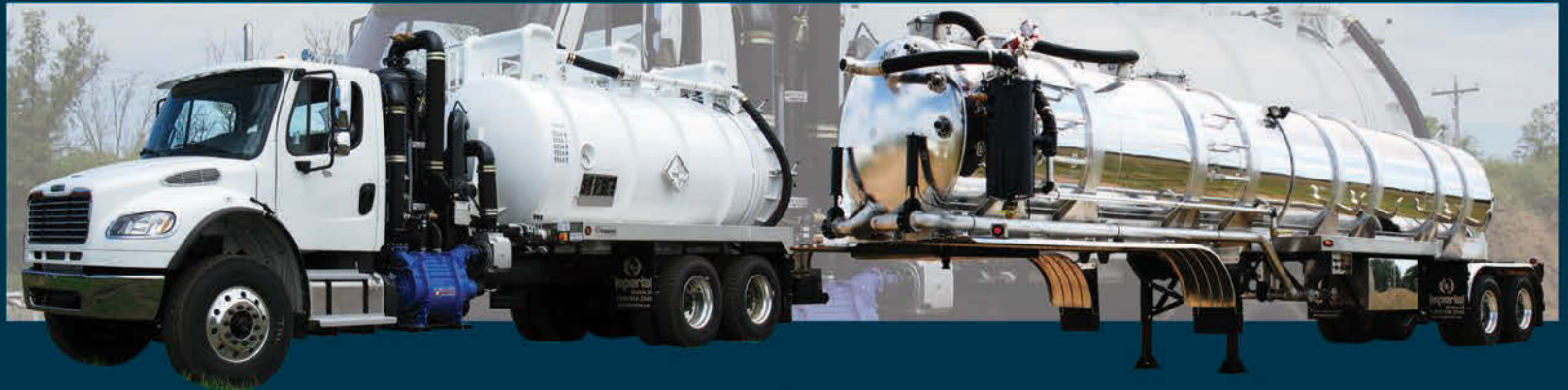
407/412 DOT Units and Aluminum Trailer Units
