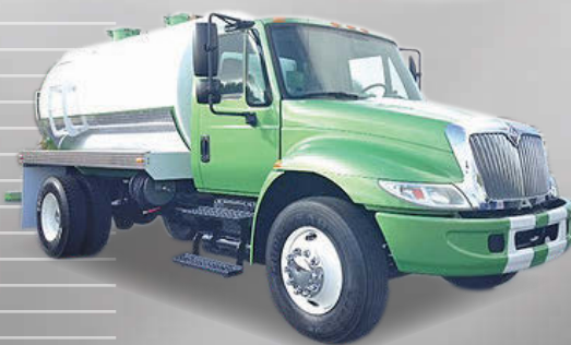
2006-07 INTERNATIONAL 4300 New 2500 Gal. U.S. Tank, DT-466, 6 SPD, Jurop R-260 9 to Choose From, $53,000
