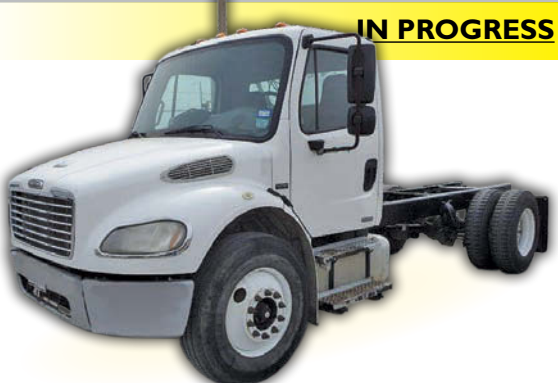
2008 Freightliner M2 , Mercedes 250 hp, Auto trans, low miles, new 2300 gallon steel vac tank, new Jurop PN-84 vac pump.
