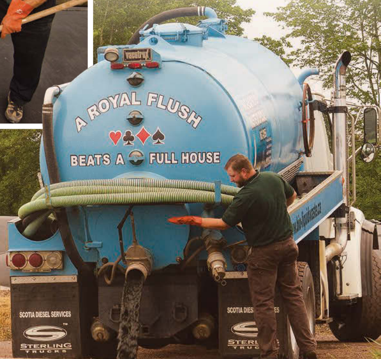
Technician Andy Ledrew dumps a 1999 Sterling vacuum truck, built out by Vacutrix, into a settling lagoon. Settled solids are transferred to geotextile dewatering tubes each fall, shown in the background.
