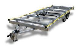
skids to be configured securely in the same load. Models range from 8 to 48 feet, accommodating up to 24 units. All models include fully independent-suspension axles that virtually eliminate side-to-side shock transfer. They are available with a front wind deflector to protect restrooms from road spray, stones and wind loading. Hot-dip galvanizing provides corrosion protection. **866/457-5425; www.explorertrailers.com.**
