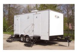
By locking an interior door, it offers a five male and one female station floor plan to be used on a male-dominated construction site. By locking a different door, the floor plan can be converted for events with three male and three female stations. It is available with onboard freshwater and a winter package. **260/593-2279; www.richrestrooms.com.**
