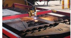
ute, and can sever metal more than 2 1/4 inches thick. The gouging system can remove more than 27 pounds of metal an hour. **800/643-0030; www.** hypertherm.com.
