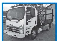
**2008 GMC W4500** portable restroom truck with Crescent tank. 39K miles. Carry 6 units; 4 on the bed & 2 on the lift gate. 550-gallon waste tank, 250-gallon fresh water tank. Thieman bar grate rail gate TVL–16 electric/hydraulic. Excellent condition ......\$42,500
