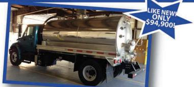
**Chassis:** 2014 International 4300, M7 Motor, 300 HP Exhaust brake, Allison auto trans **Tank:** 2500 gal alum tank with 10 yr no-leak warranty Top and rear manways, (3) 5" site eyes, LED lighting **Configuration:** NVE607 vacuum pump with hot-shift PTO, 4" discharge 3" inlet, Garnet 806(b) i gauge, heavy duty bumper
