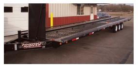
has a skid locking system that secures multiple units using an iron bar locked into place with a chain binding system. Models are available to handle from six to 20 restrooms, and all feature front deflectors to protect units from road spray and debris, brakes, paint options, lighting and leaf-spring suspension, with optional powder coating and chrome wheels. **800/498-3000;** www.cesspoolcleaners.com/johnny.html.
