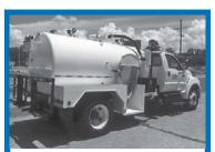
**Complete Portable Toilet service truck mount units** (turn-key), mounted on your truck or ours. Tool boxes, dual work stations, dc10 washdown pump, reversible vacuum pump, hose reel, set up complete, toilet racks available. 1100 waste/400 fresh: \$19,000, 1700 waste/600 fresh: \$20,500. Any custom options or sizes available!
