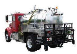
include heavy-duty tank construction, with relief set at 14.5 psi. Tanks are dual compartment with load-dampening baffles to ensure driving safety on- and off-road. They are available in carbon steel, aluminum, 304 or 316 stainless steel or 316 high-polish stainless. They come in 850- to 2,000-gallon capacities. Options include transfer pumps, heated valves, custom hose trays and toolboxes. **800/547-7790; www.vacuumsalesinc.com.**
