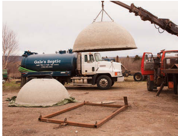
Left: Gerard Gale works the boom truck, moving a freshly made tank half at the Gale's Septic yard.
