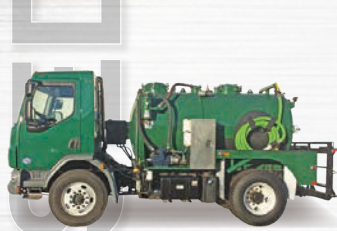
2013 Peterbilt 26,000 GVWR, auto transmission, 400/1100 stainless steel tank, Masport HXL4 pump, dual service-loaded.
