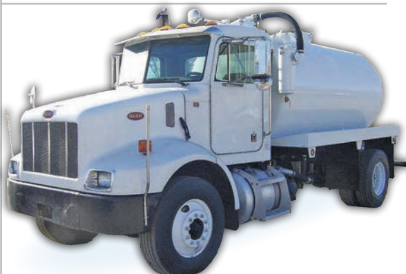
2004 Peterbilt 330 , Cat 275 HP, Allison auto, AC, low miles, new 2350 gallon steel vac tank, new Jurop PN-84 vac pump.
