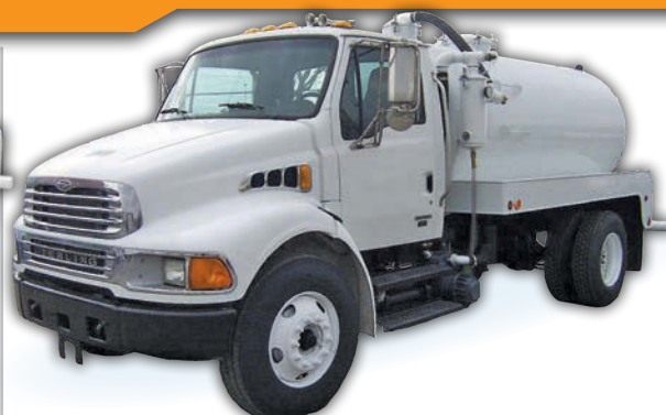
2007 Sterling Acterra , Mercedes 230 HP, 6 spd, AC, low miles, new 2300 gallon steel vac tank, new Jurop PN-84 vac pump.
