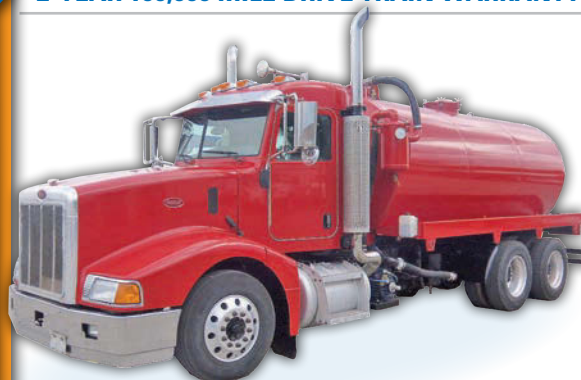
2007 Peterbilt 385 , C-13 Cat 430 HP, 13 spd, jakes, AC, new 3360 gallon steel vac tank, new liquid cooled HXL-400 Masport vac pump.
