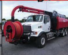
Combination Sewer Cleaner Vacall AJV 1015
