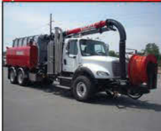
Combination Sewer Cleaner Vacall AJV 1215
