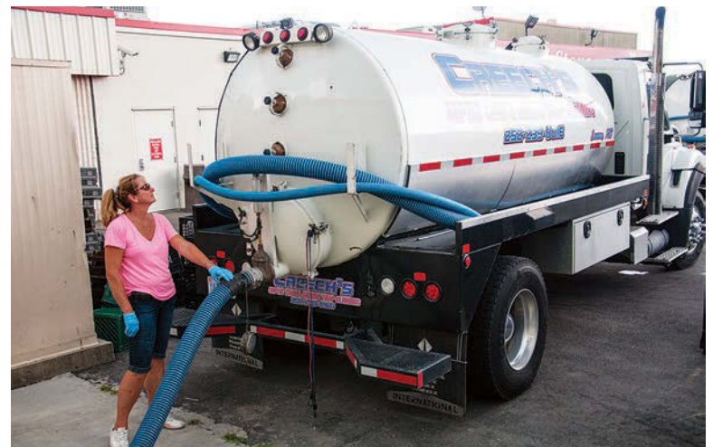
Below: Myrtle Creech makes sure everything is ready to go before pumping out another grease trap using her International WorkStar vacuum truck built out by Lely Manufacturing.
