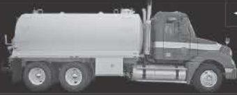
2006 Volvo, used 3100 gallon tank, new Masport HXL400WV pump
