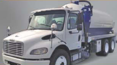
2005 FREIGHTLINER M2 New 3600 Gal. U.S. Tank, Jurop R260 Pump (363 CFM) $71,000
