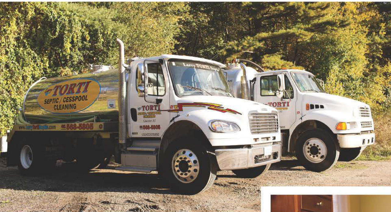
Larry Torti Septic keeps a clean two-truck fleet any single-driver operation would be proud of. His main truck is a 2012 Freightliner with 2,500-gallon Imperial Industries aluminum tank and NVE 607 pump. For backup, he keeps a 2001 Sterling Acterra with 2,500-gallon Progress VacTruck aluminum tank and Moro AC4 pump.
