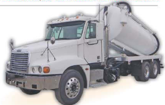
2006 Freightliner Century , Cat 430 HP, jakes, 10 spd, 14,700 lb front axle, 46# rears, new 3300 gallon steel vac tank, Full hoist, Full opening rear door, NVE 866 Liquid cooled vac pump 500 CFM, 150 gallons fresh water tank. Call For Pricing!
