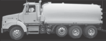
2005 Freightliner, 1600 gallon tank, Masport 75WV pump
