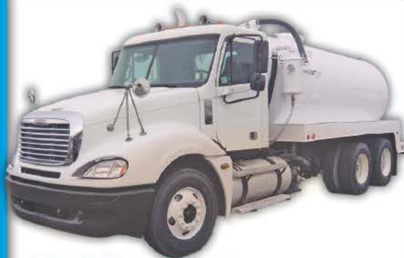
2005 Freightliner Columbia , Det. 14.0L 455HP, 10spd, jakes, double framed, low miles, new 3360 gallon steel vac tank, new Liquid cooled Masport 400 HXL vac pump. Call For Pricing!
