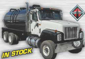
2005 INTERNATIONAL 5900, Cummins Engine, 10 Spd. New 4000 Gal Carbon Steel Tank with Masport Pump HXL40.
