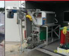
Rausch M-Series Camera Trailer • Side Office with Posm Software • Mainline & Lateral Launch • 100' Lateral Inspections • 1250' Main Cable, 6-60" Daimeter
