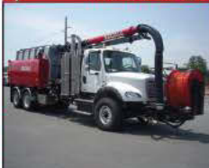
Combination Sewer Cleaner Vacall AJV 1215 • 2012 Freightliner M2 • 410 HP Diesel Engine • 85GPM @ 2000PSI Myers • Roots 18" PD Blower
