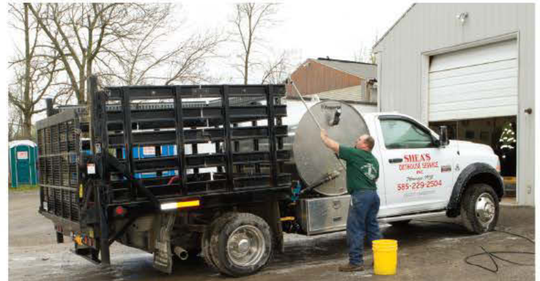
Route driver Rudy Hubble washes down his service vehicle after a day on the job. Mounted on a Dodge 5500, the truck was built out by Imperial Industries, Inc. with a 450-gallon waste tank and a flatbed to carry restrooms.
