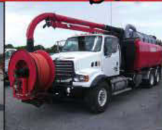
Combination Sewer Cleaner Vacall AJV 1015 • 2008 Sterling • 350 HP Cummins Diesel Engine • 80GPM @ 2000PSI GE • Roots 16" PD Blower
