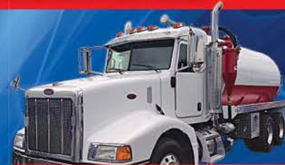
(2) 2007 PETERBILT 385 New 4000 Gal. U.S. Tank, Juropl LC-420 Liquid Cooled Pump
