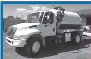
2007 International 4300: under CDL!!! Allison automatic, DT-466, low miles!! Heavy duty 2,000 gallon dual compartment U.S. tank (1,500 waste/500 fresh) with a 5-year warranty, new Jurop R260 (363 cfm) pump with a 1-year warranty, A/C, new valves and camlocks, aluminum hose trays, sight glasses, new paint, 1-year/100,000 mile engine warranty nationwide, see dealer for more details. .....$47,000
