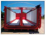
The ADS 30-yard (15-yard available), open-top, roll-off dewatering unit from Aqua-Zyme Disposal Systems can be filled with 22,000 to 25,000 gallons of wastewater treatment plant sludge, septic and/or grease trap waste at 1- to 2-percent solids in about two hours. After draining
