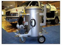
The 50-gallon Dyna-Lite portable grease pumping system from Dyna-Vac Equipment is 28 1/2 inches wide to fit through most doorways. It features a positive displacement 49 cfm vacuum pump, vacuum up to 15 inches Hg, full-opening top
