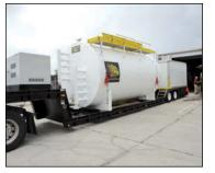
The Greasezilla brown grease separator from Downey Ridge Environmental Co. includes a 10,000-gallon (10 feet in diameter, 13 feet high and 26 feet long) insulated, double-walled horizontal reactor tank with two sets of large diameter internal heat transfer tubes, external inlet and outlet manifolds, top coffer dam with
