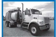
2005 Sterling AquaTech CB-10: 624 Roots PD vacuum blower. General pump, 35 gpm @ 2,000 psi, 10-yd. debris body, diesel, automatic transmission, A/C, 28,153 miles.....\$90,000 972-938-195 TX P11
