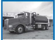
2007 Peterbilt 385 (2 available): CAT C-13 475 hp, 9-spd., 482,651 miles, new heavy duty 3,600 gallon U.S tank with a 5-year warranty, new Jurop R260 pump (363 cfm) with a 1-year warranty, heavy duty bumper, all new valves, rear work lights, new custom paint, aluminum hose trays, large 12 gallon cyclone secondary, 1-year/100,000 mile engine warranty nationwide. See dealer for more details.
