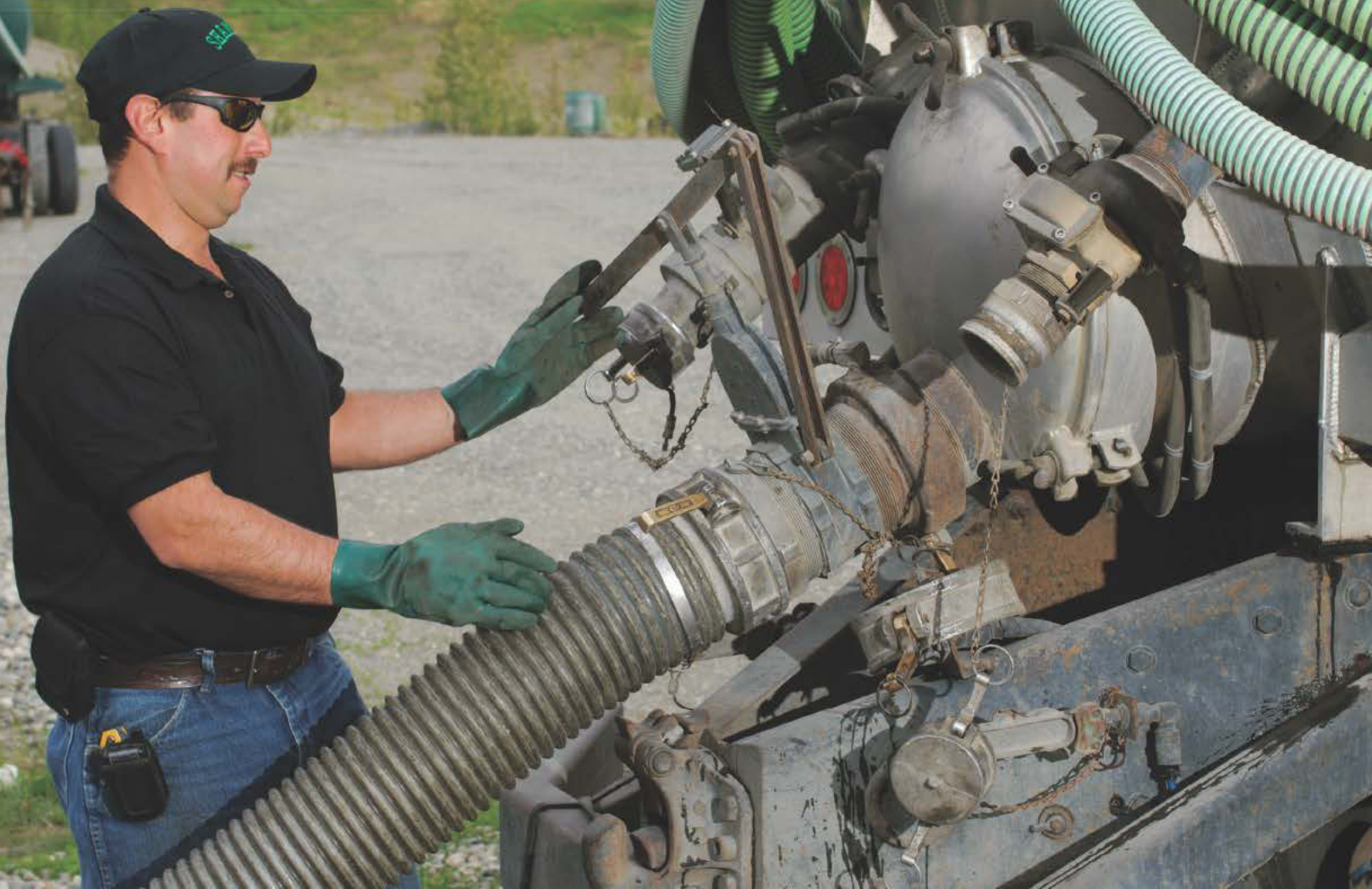
Shamrock foreman Phil Kushin empties his vacuum truck into a holding tank at the end of a day of pumping.
