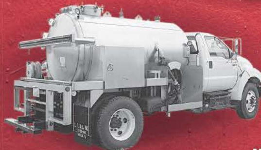
1500 Gallon 2-Compartment Stainless Steel Tank (1000/500) Mounted On 2012 Ford F750 With Masport Plug & Play Pump
