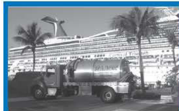
2,800 gallon PROGRESS aluminum tank: 4" front intake, 4" rear intake, 6" rear discharge. Sea Level Digital gauge. Chris Haack: 205-353-3533 P08
