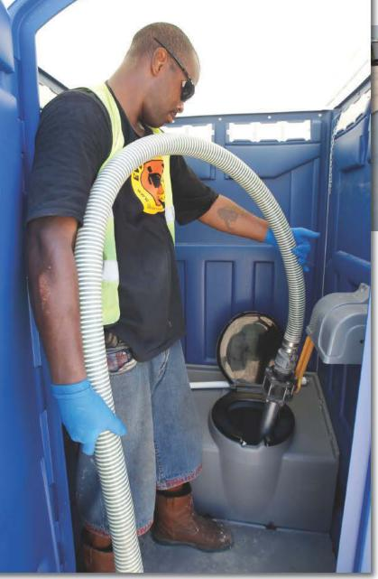
Technician Willie Dixon Jr. pumps out the holding tank of a PolyPortables restroom at Jazz Fest.
