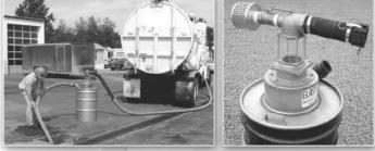
Vacuum head used to intercept liquids or solids and contain it in a 55 gallon drum. Eliminates contaminating your truck on small jobs.
