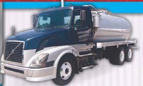
2005 Volvo VNL64T, Cummins ISX 500 HP, 10 spd, jakes, AC, double framed, low miles, **new** 3360 gallon steel vac tank, **new** liquid cooled HXL-400 Masport pump. Call For Pricing!
