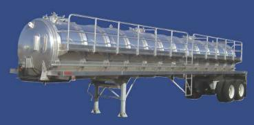
2500 Gallon Carbon Steel*Aluminum hose trays*Masport HXL15 pumping package,4" inlet, 6" discharge and 48" toolbox.
