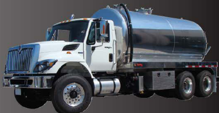
2011 International 7500 Manual transmission 3,600 Gallon Progress Aluminum 400 CFM water cooled pump system, 48" tool boxes each side.
