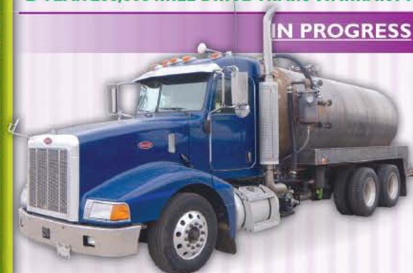
2007 Peterbilt 385 , C-13 Cat 430 HP, 9 spd, jakes, AC, new 3360 gallon steel vac tank, new liquid cooled HXL-400 Masport vac pump.
