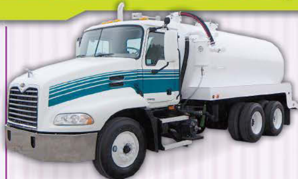
2004 Mack CX613 , AI-350 HP, 10 spd, jakes, AC, double framed, new 3360 gallon steel vac tank, new liquid cooled HXL-400 Masport vac pump.
