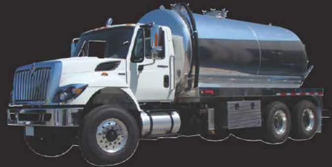
2011 International 7500 Automatic transmission 3,600 Gallon Progress Aluminum 400 CFM water cooled pump system, heated inlet and discharge with 48" tool boxes each side.
