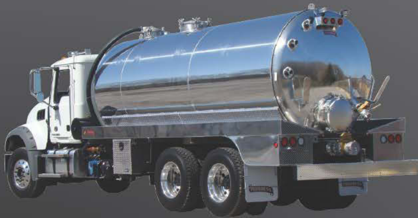
Mack GU433 4200 Gallon Progress Aluminum Tank Robuschi RB-DV45 Blower Package • 500 CFM
