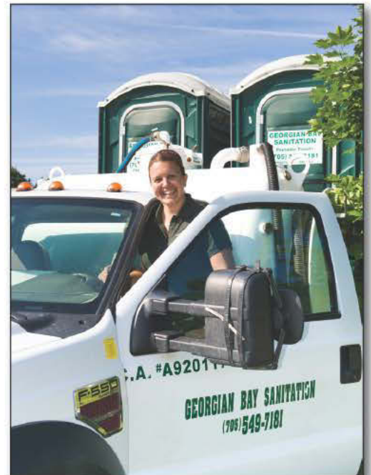
Laurie Robillard prepares to deliver another load of restrooms with her 2001 Ford F-550 with a 350-gallon waste/200-gallon freshwater Vacutrux slide-in unit.
