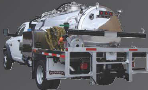
2011 Dodge 5500 4x2 1,250 Gallon Progress Pro Series Tank Masport HXL4V
