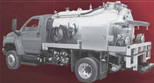
1350 Gallon Stainless Steel Portable Restroom Service Truck Mounted On 4x4 Chassis
