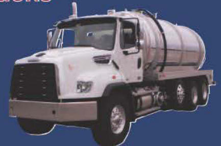
2012 Freightliner 114SD 4800 Gallon Aluminum Tank Masport VTK-650
