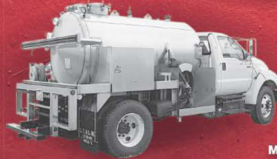
1500 Gallon 2-Compartment Tank (1000/500) Mounted On 2012 Ford F750 With Masport Plug & Play Pump
