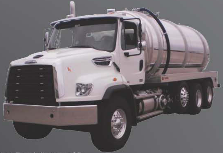
2012 Freightliner 114SD 4800 Gallon Aluminum Tank, Masport VTK-650
