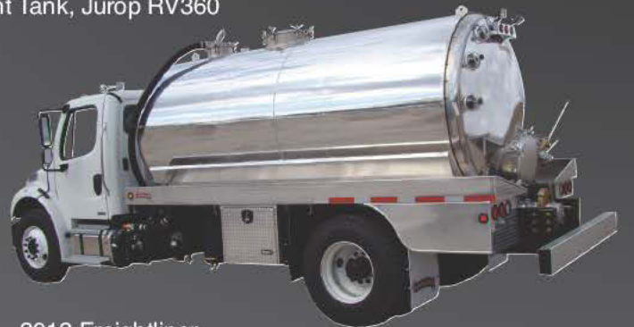
2012 Freightliner 2800 Gallon Aluminum Septic Tank, Masport HXL 15
